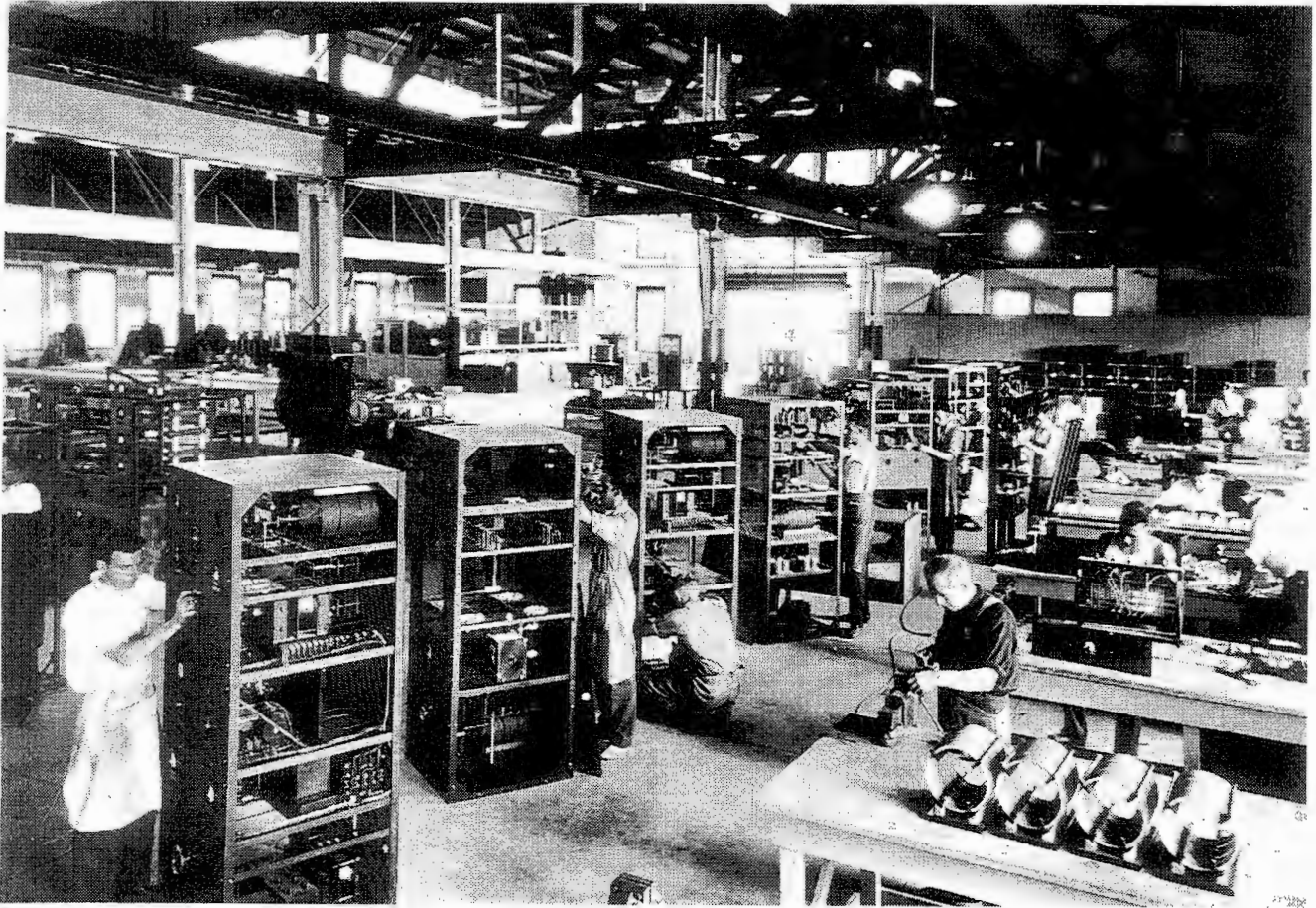
Radio transmitters being built at AWA's Radio-Electric Works at Ashfield, Sydney, in the mid-1930's. Many of the transmitters used by the first generation of Australia's radio broadcasters were built in this factory. (Courtesy AWA).
