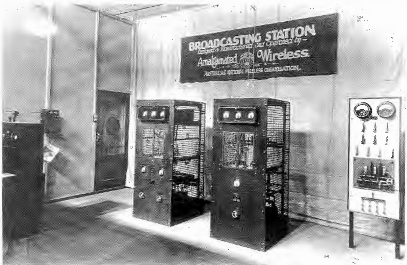
An early AWA broadcasting transmitter, designed and manufactured in Australia, on display in the late 1920's. The picture was probably taken at AWA's Melbourne offices. (Courtesy AWA).
