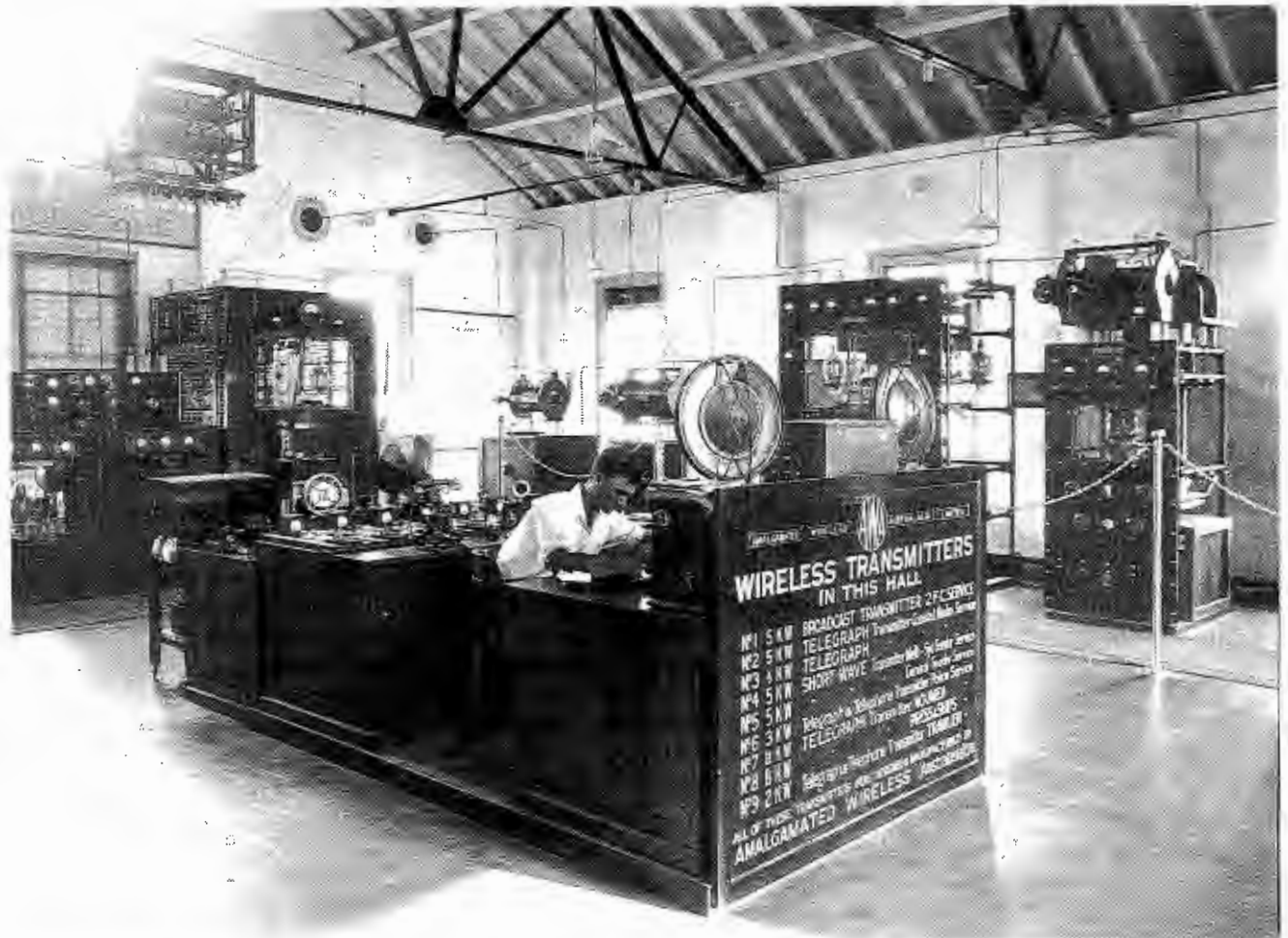
Part of the AWA transmitter hall at Pennant Hills, in 1927. The sign on the front of the operator's desk explains that by that stage, there were eight other transmitters housed in the hall apart from the 5kW transmitter for 2FC. Apart from two 5kW shortwave units used for broadcasting feed interstate, the rest were mainly used for telegraph and telephone links. (Photograph by courtesy of AWA).
